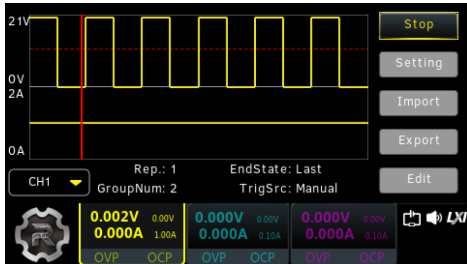
Figure 9.5 Arb Output Interface
